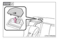
Remove the anchor bracket cover.
