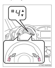
Temporary manual mode driving can be changed to by operating the paddle shift levers while the select lever is in the D position.
