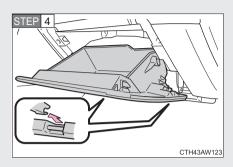
Pull out the glove box and disconnect the lower claws.
