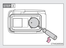
Remove the depleted battery.
