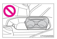
When placing the cup holder, make sure it is facing the correct direction. Failure to do so will cause the cup holder to not be secure in the console trav and hinder select lever or shift lever operation.
