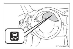
The slip indicator light will flash while the TRAC (brake LSD function)/Vehicle stability control (VSC) systems are operating.
