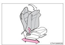
Lift the seatback angle adjustment lever.
