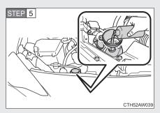
Add engine coolant if necessary.
