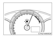
When the set engine speed is reached the REV indicator comes on and a buzzer sounds to inform the driver.  $(\rightarrow P. 197)$
