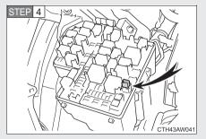
Remove the fuse with the pullout tool.
