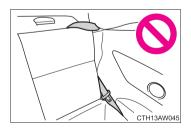
Always make sure that the seatbelt is not caught in the seatback or twisted in one of the hooks that secure the seatback. Failure to do so may cause the seatbelt to not be fastened correctly or to become ineffective in a collision, resulting in serious injury.
