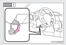
Hold the steering wheel and push the lever down.
