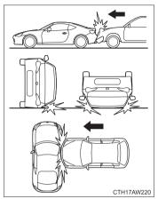
The driver's and front passenger's SRS frontal airbags are designed not to deploy in most cases if the vehicle is struck from the side or from behind, or if it rolls onto its side or roof, or if it is involved in a low-speed frontal collision.
