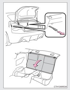
Pull the both left and right seatback lock release straps in the trunk lid to fold down the seatback.
