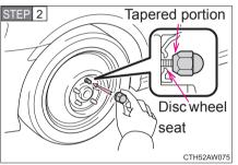
Install the spare tire and loosely tighten each wheel nut by hand to approximately the same amount.
