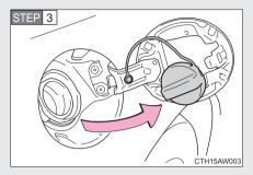
Hang the fuel tank cap on the back of the fuel filler lid.
