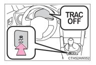
Press  $\left|\begin{array}{c} \frac{2}{6\pi} \end{array}\right|$  to turn off TRAC. ( $\rightarrow$ P. 216)
