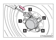
After installing "A" as shown in the illustration, push the center ornament claws in the order shown in the illustration using a flathead screwdriver.
