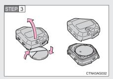
Open the case cover using a coin protected with tape and remove the depleted battery.
