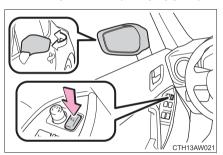
Press the switch to fold the mirrors.
