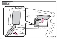
Open the cover and remove the lens.
