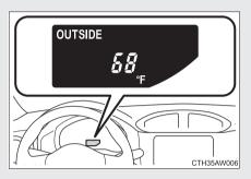
The outside temperature display can be switched by pressing the "DISP" switch.  $(\rightarrow P. 196)$
