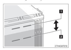
Check that the level is between "UPPER LEVEL" and "LOWER LEVEL".
