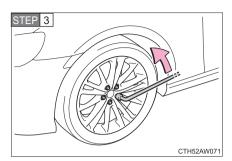
Slightly loosen the wheel nuts (one turn).
