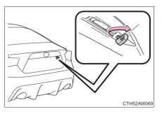
Turn the mechanical key clockwise to open.
