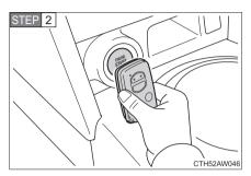
Touch the SUBARU emblem side of the access key to the push-button ignition switch.
