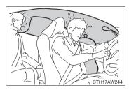
The SRS side airbag and SRS curtain airbag can function only when the ignition switch is in the "ON" position.
