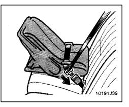
Run the lap and shoulder belt through or around the infant seat following the instructions provided by its manufacturer and insert the tab into the buckle taking care not to twist the belt. Keep the lap portion of the belt tight.
