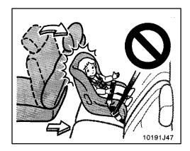
• Do not use a rear-facing child restraint system in the rear seat if it interferes with the lock mechanism of the front seats. This can cause severe injury to the child and front passenger in case of sudden braking or a collision.
