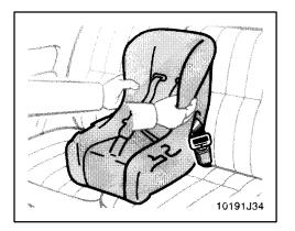
Push and pull the child restraint system is different directions to be sure it is secure. Follow all the installation instructions provided by its manufacturer.
