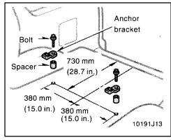
If your child restraint system requires the use of a top strap, latch the hook onto the anchor bracket and tighten the top strap.
