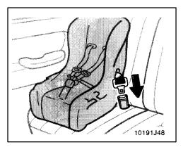
1. Run the lap and shoulder belt through or around the convertible seat following the instructions provided by its manufacturer and insert the tab into the buckle taking care not to twist the belt. Keep the lap portion of the belt tight.
