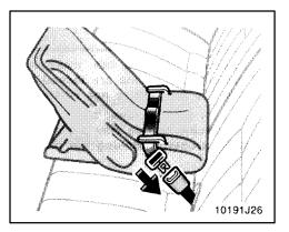
1. Run the center lap and shoulder belt through or around the infant seat following the instructions provided by its manufacturer and insert the tab into the buckle taking care not to twist the lap belt.
