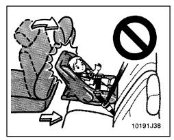
• Do not put a rear-facing child restraint system in the rear seat if the child restraint system interferes with the front seat lock mechanism or with your proper driving position. This can cause severe injury to the child and front passenger in case of sudden braking or a collision.
