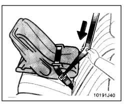
2. Fully extend the shoulder belt to put it in the lock mode. When the belt is then retracted even slightly, it cannot be extended.
