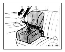
2. Fully extend the shoulder belt to put it in the lock mode. When the belt is then retracted slightly, it cannot be extended.
