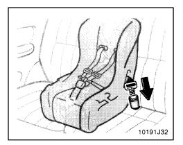
Run the center belt through or around the convertible seat following the instructions provided by its manufacturer and insert the tab into the buckle taking care not to twist the lap belt.
