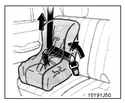
3. While pressing the convertible seat firmly against the seat cushion and seatback, let the shoulder belt retract as far as it will go to hold the convertible seat securely.
